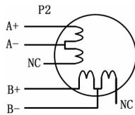
Figure 6: 6-lead motor half coil (higher speed) connections
