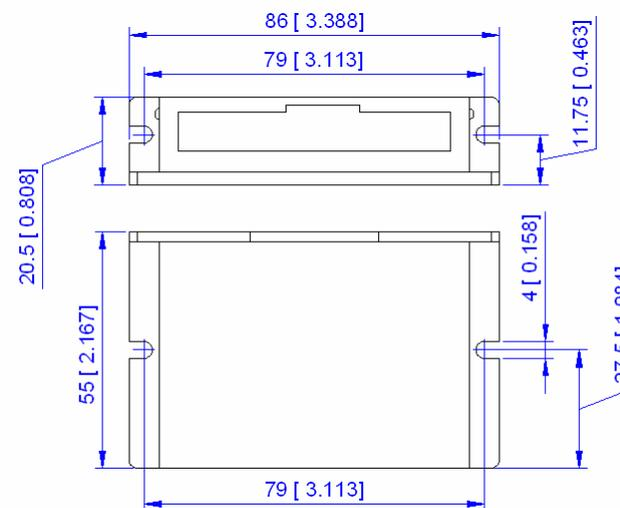
Figure 1: Mechanical dimensions
