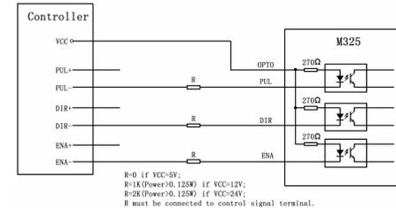
Figure 4: Connections to difference control signal
