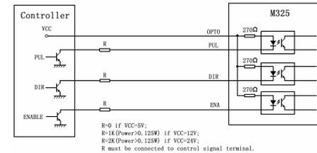
Figure 3: Connections to open-collector signal (common-anode)
