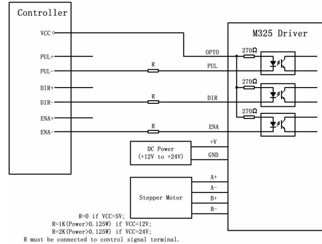
Figure 11: Typical connection with difference controller
