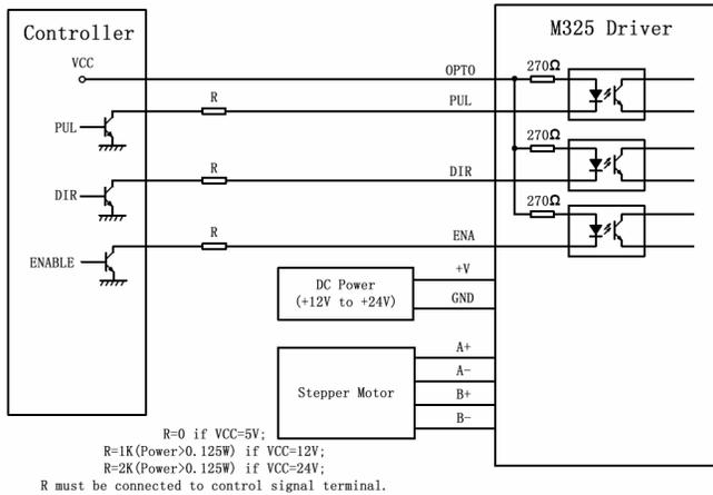
Figure 10: Typical connection with open-collector controller
